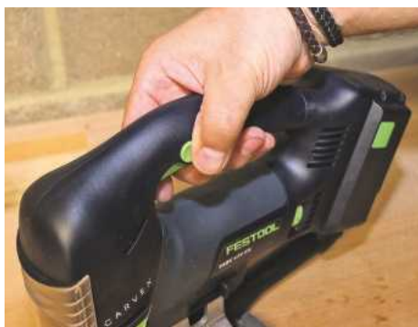
▲ The hoop handle has a variable-speed trigger for normal work
